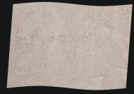
granulation: 0 ÷ 1 mm layer thickness: 3 ÷ 4 mm
